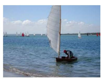
professional sailmaker, put together a replica of the rig used on the 1950s boats which had a curved gaff for the gunter cat-rigged sail. The narrow panels on the sail make it highly authentic.
