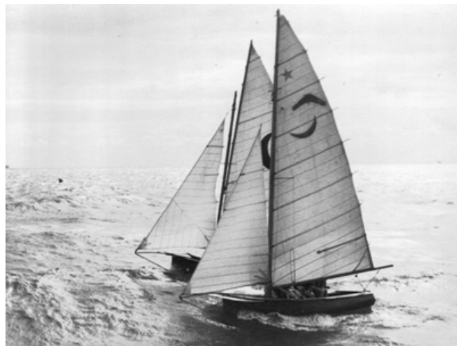
Right Mick and Noel Brooke trialling a 'Marconi' rig and gunter rigged skiffs on Port Phillip Bay. The newer sloop rigs used a lot of stays and spreaders so were termed Marconi's because the masts looked like radio towers.
